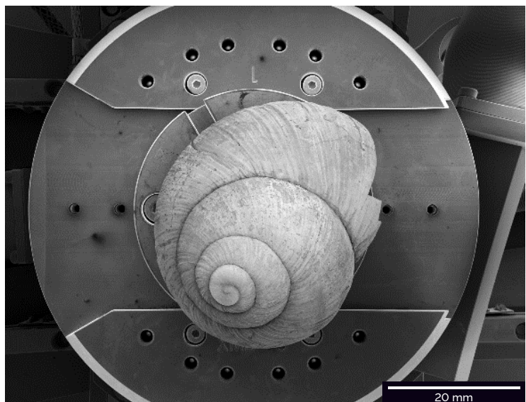
▲ Snail shell ( Helix pomatia ) on the SEM stage captured with SE detector. Field of View is >8 cm (>3 inches).
